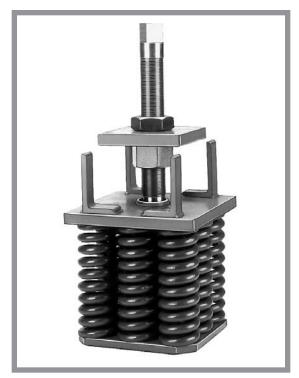
A heavy duty spring isolator most frequently used to support machines on deep concrete foundations such as forging hammers and roll grinders. The structural members cast through the foundation are supported by the UN isolator, and machine and foundation is levelled through adjustment of the isolator. Separate snubbing and damping controls are available. Load range to 35,000 lbs. per isolator and deflections to  $1\frac{1}{2}$ " result in excellent shock and vibration attenuation.
